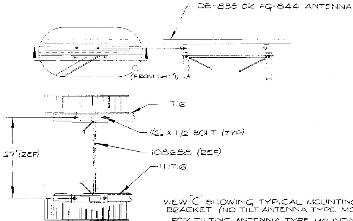
VIEW C SHOWING TYPICAL MOUNTING OF ANTENNA TO BRACKET (NO TILT ANTENNA TYPE MOUNTING); FOR TILTING ANTENNA TYPE MOUNTING SEE SHEET #4
