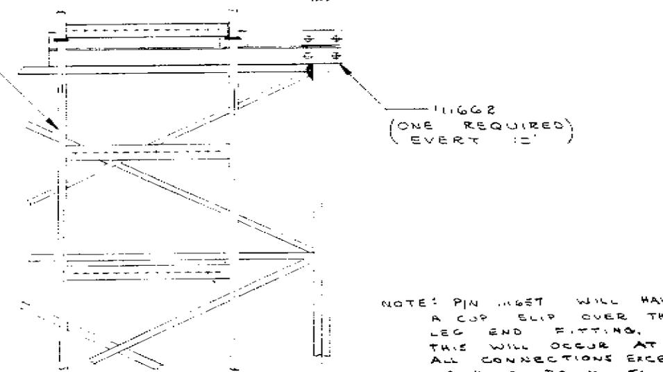
NOTE: PIN JOIST WILL HAVE A COP SLIP OVER THE LEG END FITTING. THIS WILL OCCUR AT ALL CONNECTIONS EXCEPT THE KNOCK-DOWN TO FABRICATED INTERFACE. THIS CONNECTION WILL BE A LOOSE CONNECTION.
